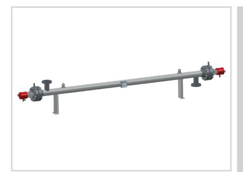
Electric heat exchangers to heat liquid or aeriform fluids with varying pressure up to 300 bar. Used in cases of high differences in inlet and outlet temperature and in cases of installations requiring a high energy input. Designed with a single vessel on which a heater is installed on either side. The reason for a dual head is to limit the temperature on the surface of the heaters as a consequence of a wide range of variation of process temperatures.
